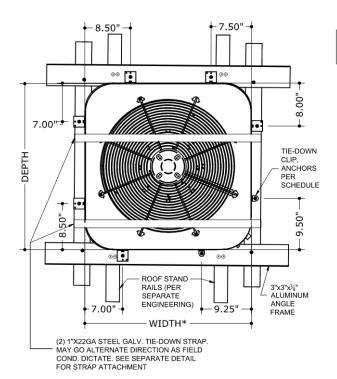
\*NOTE: FOR CONDITIONS WITH STAND DEPTH GREATER THAN UNIT DEPTH, MIAMI-TECH SUPPORT ANGLES (PART #AS14CABBXX) PER NOA#17-1218.02 SHALL BE PROVIDED OR SITE-SPECIFIC ENGINEERING IS REQUIRED.
