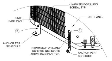
**TIE-DOWN CLIP** 2" WIDE AND 4" TALL MIN ASTM A653 14 GA GALVANIZED STEEL. FASTEN CLIP TO HOST STRUCTURE USING ANCHOR FROM "ANCHOR SCHEDULE TO HOST STRUCTURE" TABLE AND (1)#10-16 X  $\frac{1}{2}$ " SS316 MIN SELF-DRILLING SCREWS TO FASTEN CLIP TO UNIT
