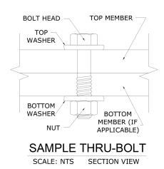
Note: The term "Thru-Bolt" or through bolt, if used herein, refers to a bolt passing through the member(s) in contact and is fastened by a nut at the end opposite the screw head. Nut shall be equivalent to or exceed the strength of the bolt U.N.O. Nut shall be sized to accommodate the same nominal diameter as the bolt U.N.O. See diagram above-right for a sample thru-bolt configuration.
